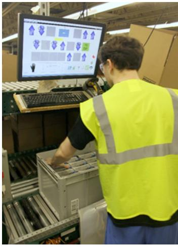
The goods-to-person workstation includes an operator interface monitor to display picking instructions.
