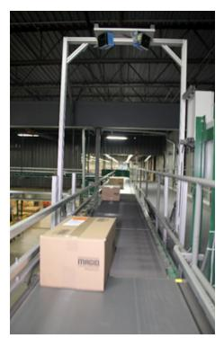
The scan tunnel reads barcodes on each carton.
