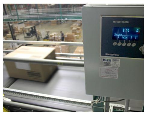
The in-line scale weighs each carton on-the-fly.
