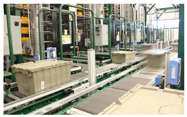
Multishuttle In/Out Conveyor Loop: Connects the Multishuttle to the workstations. Inventory totes are brought to and from workstations.
