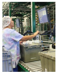
**Workstation:** Workers interact with Dematic software user interface to confirm assembly process.
