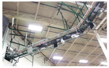
**Overhead Conveyor:** Gray totes with inventory flow from manufacturing to the assembly area via overhead accumulation conveyor.
