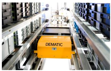
**Multishuttle Work-in-Process Buffer:** Inventory totes are stored in this Multishuttle sub-system until needed at assembly workstations.
