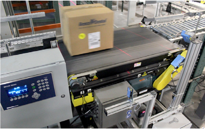
Order cartons are weighed “on-the-fly” prior to shipping.
