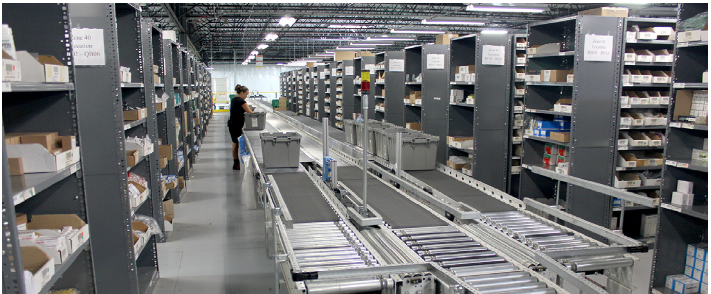
The center conveyor is an expressway though to the pick module. Order totes are transferred to the sidings if a pick is required in that zone.
