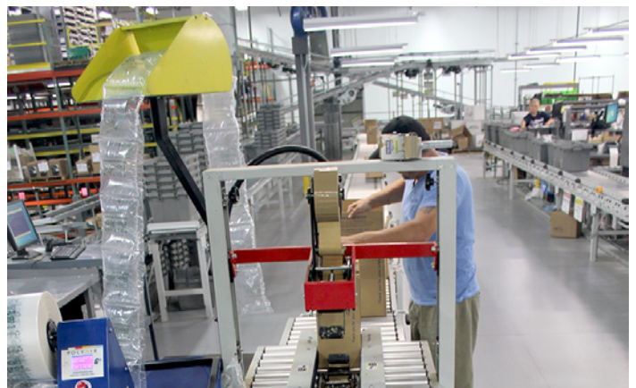
Void fill is added prior to case sealing.
