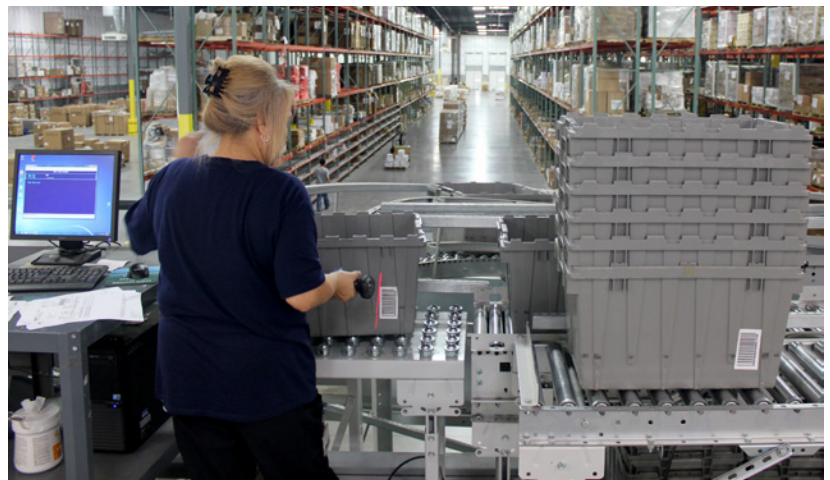
Order totes are scanned at the order start workstation.
