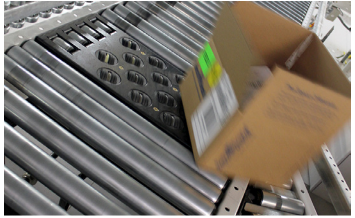
The steerable wheel sorter diverts order cartons prior to case sealing.
