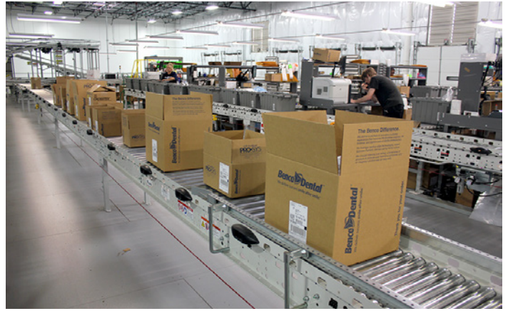
Order containers are in queue at the case sealer workstation.
