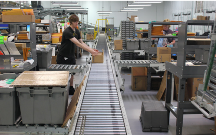
After packing, the order cartons are conveyed to the case sealer.
