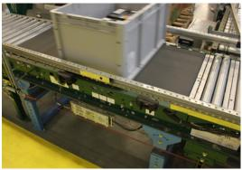
Each inbound inventory tote passes over an in-line weigh scale to confirm and verify stock keeping unit count.
