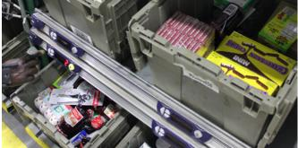
At the order assembly workstations, light-directed technology indicates the totes for operators to "put" the items. The slot display shows the quantities.
