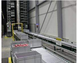
The conveyor network connects the workstations with the Multishuttle.
