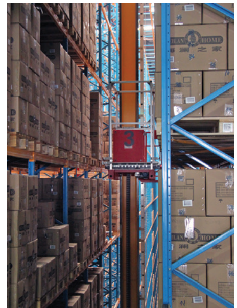
89 ft high ASRS with 73,200 pallets
