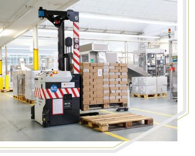
The AGVs are not necessarily faster, but they perform the tasks smoother and safer. On average an AGV takes about eight minutes to transport a pallet with packaging materials from the warehouse to the production line.
