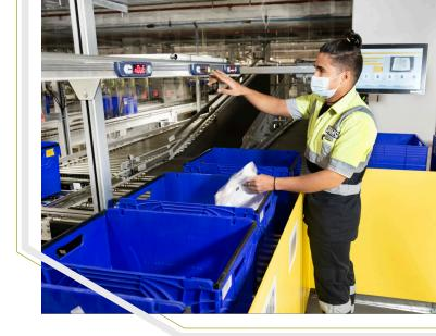
580,000 storage places. The daily requirement of a good 370,000 items is retrieved with the help of 528 Dematic Shuttle Static units in the adjacent Dematic Multishuttle on 24 levels. In this way, up to 15,000 totes per hour can be transported to the picking stations. By using a total of 94 lifts as well as shuttles controlled via power rails with very high acceleration and speed performance, one shuttle can operate between 700 and 800 storage spaces.
