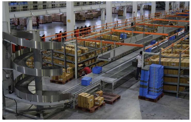
A Spiral Conveyor transfers orders from the Mezzanine to the Pick-to-Light system. Global induction enables orders to start in the first zone where items are required for an order, reducing order assembly time and improving order picking efficiency.
