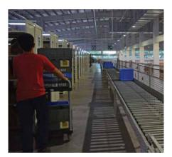
In the shelving area, picking is directed and confirmed by operators using hand-held wireless terminals.
