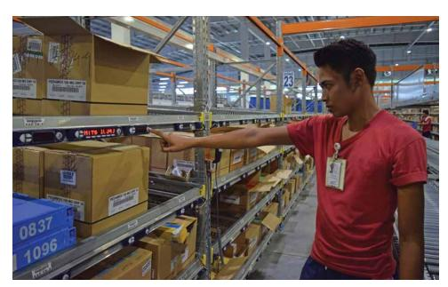
Stock locations in the PTL system are fitted with a digital readout indicating the quantity of items to be picked for each order, enhancing accuracy.
