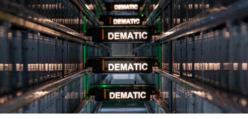
As part of the solution, Dematic set up a Dematic Multishuttle® automated storage and retrieval system. Products are placed in open totes, which are then stored in high-density racks. The system selects the best storage locations and shuttles automatically transport the incoming totes to designated rack locations. These towering racks reach the ceiling of the main storage floor, maximising the storage density of the warehouse.
