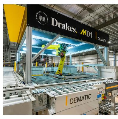
The GTP Picking Solution delivers items directly to pick stations – eliminating the need for operators to spend time manually locating and retrieving items and travelling across the DC floor. The solution focuses on the challenging aspects of fulfilment by combining high-density secure storage with the rapid rate and high accuracy of directed picking, equipped with an ergonomic design to enhance operator performance.
